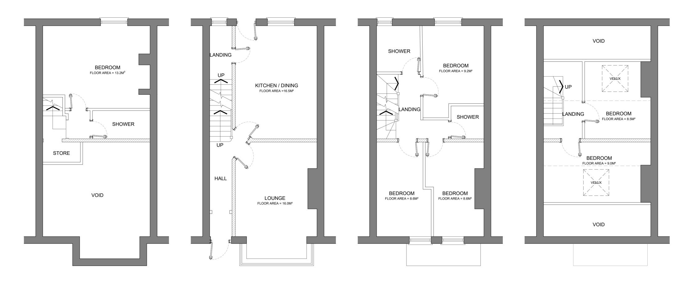
LOWER GROUND FLOOR PLAN GROUND FLOOR PLAN FIRST FLOOR PLAN SECOND FLOOR PLAN
